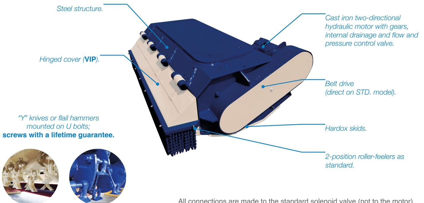
All connections are made to the standard solenoid valve (not to the motor).
