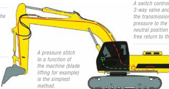
A free return to the tank is recommended (in any case max 2 bars counter pressure).
