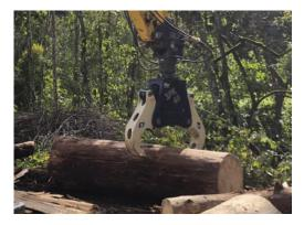
The clamp allows the wood to be processed anywhere and in any conditions directly on the ground, with the possibility to perform all handling operations using the clamp itself.
