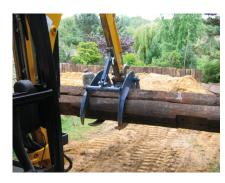
The upper jaw, activated by the cylinder closes, blocking by this way the two bodies .
