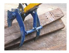
The lower jaw is connected to the machine's arm by a connecting rod. The upper jaw, activated by the cylinder, closes on the body to be moved.
